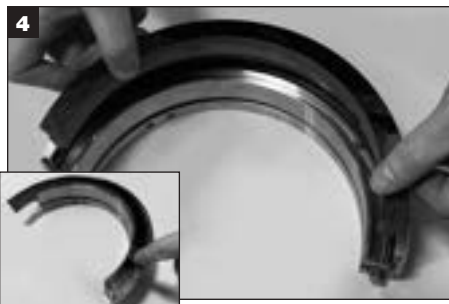
4 Remove rotary face halves (2x) by pushing on end of face and sliding out of rotary holder half. On the half with the lug, lift out the rotary seal ring, do not try and push as the seal ring will break.
