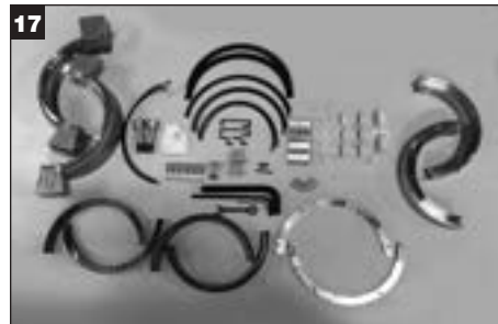
Remove all spare parts kit components from packaging and place on the clean work surface.
