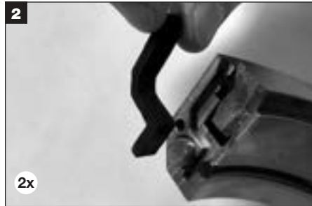
2 Remove rotary holder gaskets.
