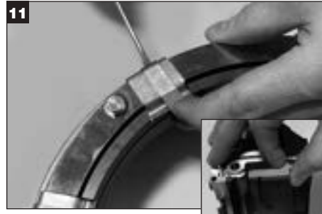
Remove (6x – 8x) spring retainers from gland halves. Note: When last retainer is removed the stationary seal ring can be removed.
