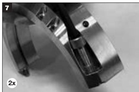
7 Remove holder cap screws from holder halves.
