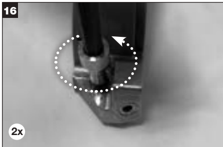
Remove gland cap screws. Ensure the gland, holder, and spring plate are free from debris, grease, and damage.
