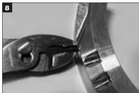
8 Remove centering buttons from (6x) outside diameter of rotary holder.
