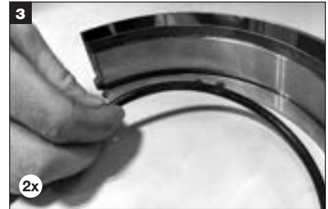
3 Remove shaft O-Ring halves.
