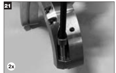
Lubricate threads with a recommended anti-seize compound and install holder cap screws in rotary holder half.
