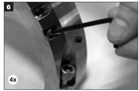
6 Remove holder set screws from rotary holder.
