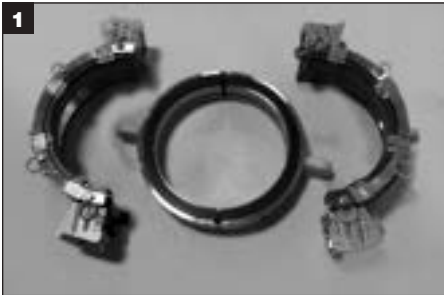
1 Prepare a clean work surface for seal disassembly and rebuild.
