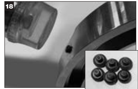
Install new centering buttons (6x) on outside diameter of rotary holder. Important: Make sure buttons are fully seated without deforming or cracking the exposed heads.
