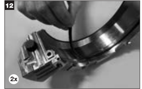
Remove stationary O-Ring halves.
