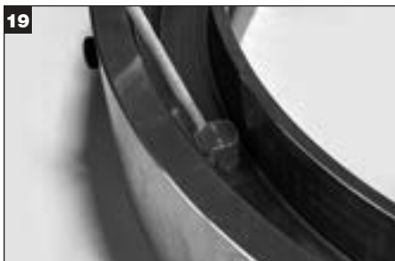
Pick up the drive tube (use tweezers if necessary) and install onto the holder lug. Ensure the drive tube is fully seated on the lug.
