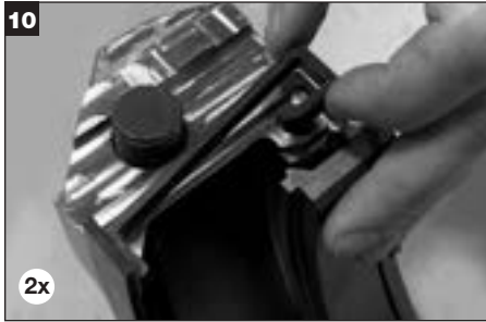
Remove gland gaskets from gland grooves.
