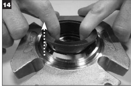
Remove the outboard stationary seal ring from gland and discard.
