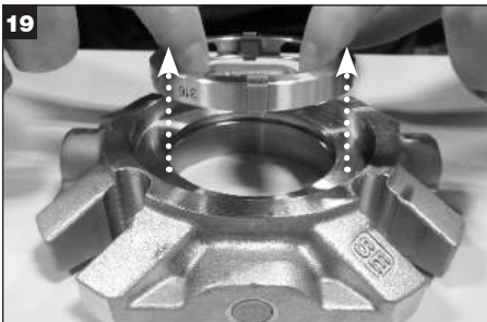
Remove the drive channel from gland; remove the channel clips and the flow deflector from the channel and discard.
