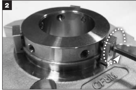
Remove the centering clips and discard.
