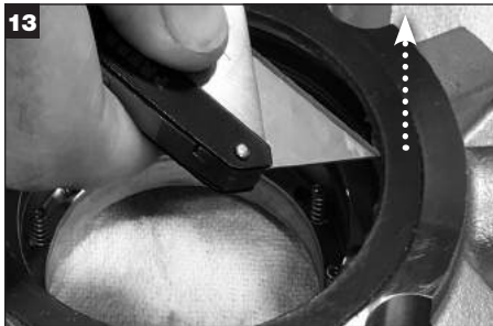
13 Remove the stuffing box face gasket from the gland and discard.
