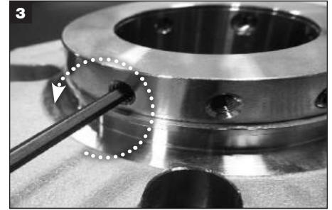
Remove all cup point and 1/4 dog set screws from the lock ring and discard.
