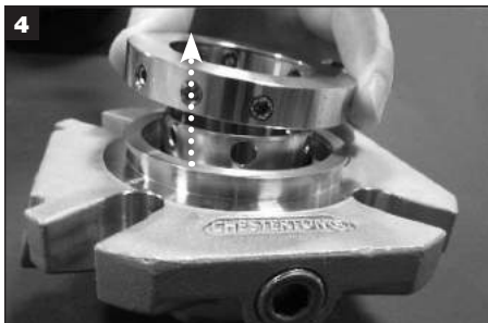
Remove the lock ring from sleeve and set aside.
