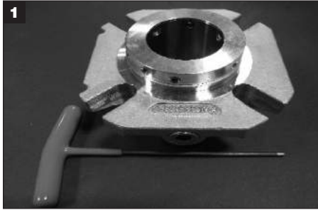
Tools required for disassembly of seal: Hex key (supplied with seal); tweezers and a curved pick (supplied by customer; for removal of O-Rings and drive tube).
