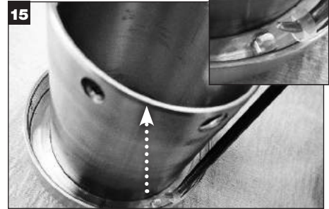
15 Remove drive from drive lugs in the sleeve and discard.
